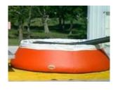
Upon arrival at the fire site, we will deploy a 500-gallon portable low-sided water tank with a floating rim as illustrated at left. It can be filled with seawater at a rate of 30-90GPM (subject to elevation). The presence of the tank will allow pumps carried in the 1<sup>st</sup> Response Trailer to draw from it and each lay water or foam on the fire at rates of 15 or 30GPM (as appropriate). This arrangement is designed for continuous operation.
